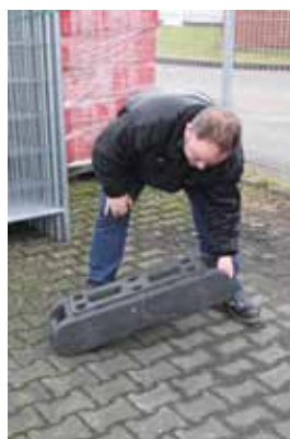
Base plate for site fences type 2 to carry with one hand because of 2 handles
